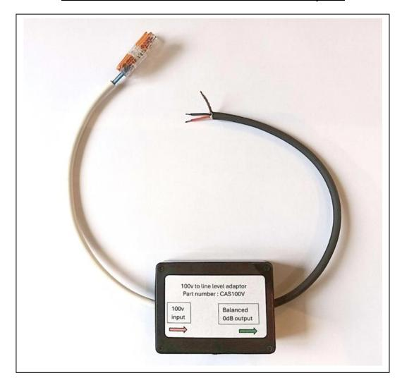
100v line to line level adaptor, transformer isolated.
